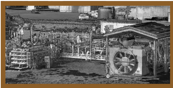
3D point cloud by LuxGear and visualized in LuxWeb
